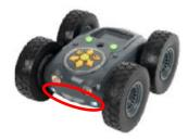
If the headlights are already off, you can make Tuff-Bot think it is dark by placing a finger over the light sensor. Then the headlights will turn on. Try it!
