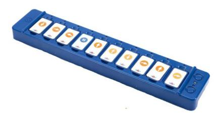
You can place up to 10 tiles in the slots. A small light turns on when the command is being run. Did you put the commands in wrong? It's easy to fix your code! Just switch the tiles around or add different ones. Press the Send button to try your program again.
