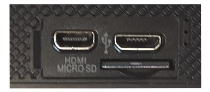
Insert the card so that the contact bars are toward the front of the camera. Slide it in all the way. If you need to remove it, just push on it and it will pop out.
