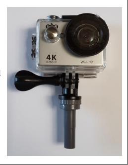
Now you need to insert the Micro SD memory card. To do this, you need to remove the waterproof casing. Pull up on the black hinged latch closest to the lens on the front of the camera. It may take a bit of force to open it. Lift up the back end of the hinged latch to open the casing. Now you can extract the camera.
