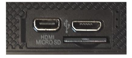
Insert the card so that the contact bars are toward the front of the camera. Slide it in all the way. If you need to remove it, just push on it and it will pop out.
