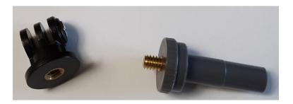
Unscrew the knob of the currently attached mount and remove the part that was screwed to it.
