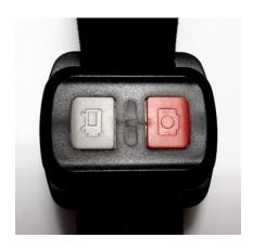
Turn the camera on by pressing the Power button on the front. Place the mounted camera in the center hole of robot and start recording. Either use the wristband remote or press the Select button at the top of the camera. You will use the same button to turn off recording.
