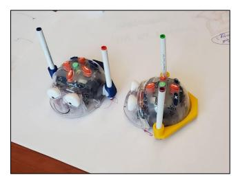
Figure 2. Bee-Bots with 3D printed attachment that holds two markers.
